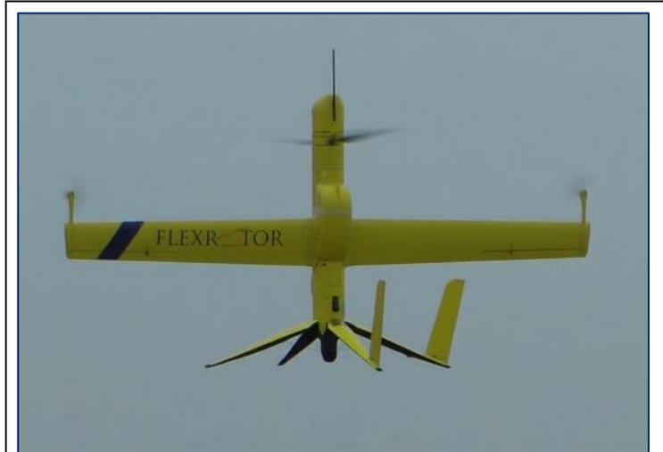
*Actaea* lifts off into gray and rainy skies at the start of its 32-hr flight. Legs are about to fold for transition to wing-borne flight.
